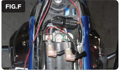
10 Plug the PCV in-line of the ignition coil and stock wiring harness.
