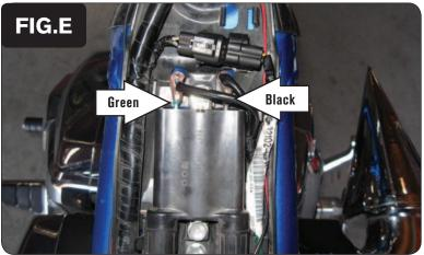
9 Locate the Ignition coil under the fuel tank. Unplug the stock wiring harness from the ignition coil paying attention to the wire colors.
