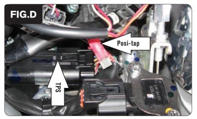
8 Using the supplied posi-tap connect the GREY wire of the PCV to the RED/YELLOW wire of the stock Throttle Position Sensor (Fig. D).
