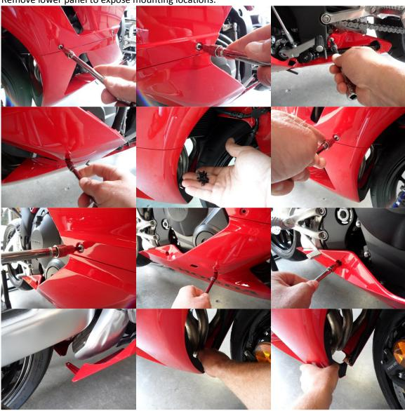
NOTE: There are tabs that help align the lowers with the mid-section. DO NOT force the lowers to come off this can cause the tabs to break off.
