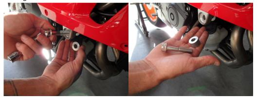
6. Line up the edge of the offset (wile mounted) with the edge of the frame and torque down to OEM torque specs using the stock OEM 12mm Hex Flange bolt. Make sure that the coolant line is secure, routed properly and is not being pinched by the offset or clutch cable in anyway.
