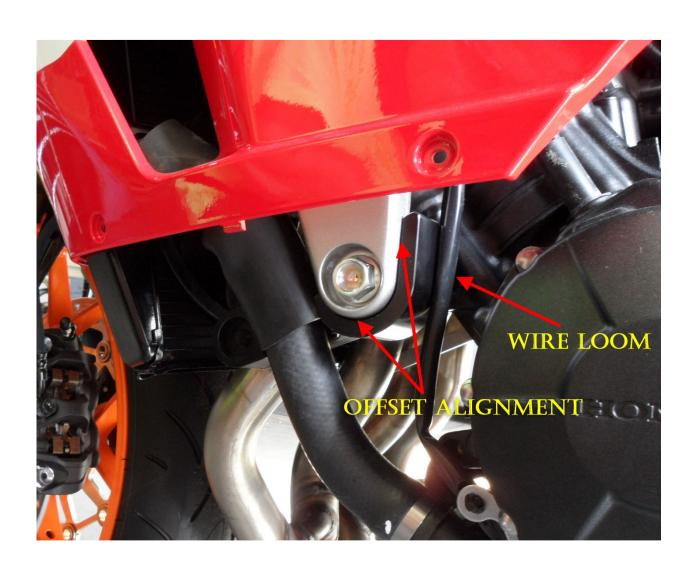
4. With the offset now aligned and torqued down adjust the coolant hose sleeve down enough to cover the coolant hose where bodywork (upper sec.) and offset meet the hose.
