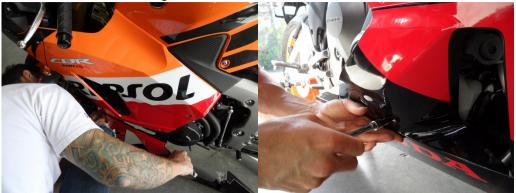
8. On the left side use one drop of blue thread locker on the (99-HB-SH10125080) Socket Cap 10 X 1.25 X 80 (Holds puck to offset). Torque down to 30 to 32 foot lbs. On the right side use one drop of blue thread locker on the (99-HB-SH10125070) Socket Cap 10 X 1.25 X 70 (Holds puck to offset). Torque down to 30 to 32 foot lbs.
