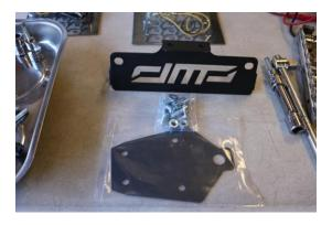
9. Mount the base bracket using two 6x1.0x12 bolts with two 6x12 (smaller) washers (medium thread locker is recommended).
