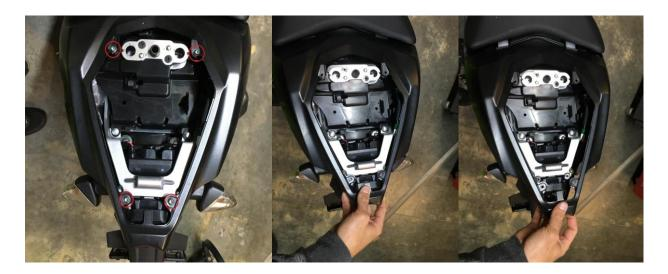
4. Pull out the foam block (let it hang). Remove the relays from the plastic relay bracket. Unbolt and pull aside the plastic relay bracket to expose the turn signal harness (DO NOT UNPLUG THE CONNECTOR CIRCLED IN RED).
