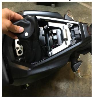
3. Remove the four bolts circled in red and remove the top portion of the tail section bodywork.
