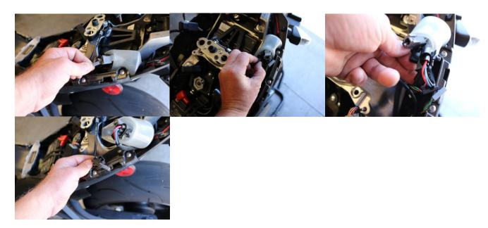
7. Remove the four bolts holding the stock fender. Remove the stock fender and guide the wires through the center of the under tail.
