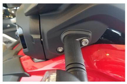
Remove the OEM fasteners at the turn signal stocks on both left and right turn signals. The rear fastener is removed using a T30 bit and 10mm spanner to hold the nylock nut in the rear. These will be reused. The rear fastener is removed with a T25 bit. This fastener will be replaced. Twist turn signal stock one quarter turn to remove.
