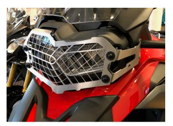
Insert (4) rubber grommets into steel mesh or lexan headlight guard lens. If needed, use a touch of water on the grommet to lubricate.
