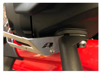
Insert turn signal stock through the bracket, and rotate into the correct position as shown. Insert M5 spacer in between bracket and headlight assembly, and secure with M5 fastener in the forward hole location with M3 driver. Resecure T30 fastener while holding the rear nut with a 10mm wrench. Hand tighten fasteners until secure. Repeat on both sides.
