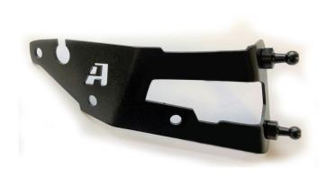
Install the (4) custom ball studs into the right and left side brackets. Add a drop of thread locker and hand tighten. hold the ball studd with 10mm spanner and turn M4 fastener with 2mm hex key. Be careful not to heavily torque the small M4 fastener.
