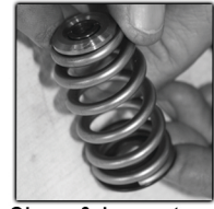
Clean & Inspect new springs & hardware
