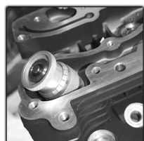
Measure spring installed height and seal to retainer clearance. Proper clearance from coil bind is critical.
