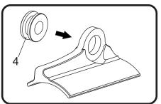
7. Install (No. 7) ALS-047 for Husqvarna OR ALS-056 for KTM, aluminum spacer in the backside of (No. 4) Z1023, rubber grommet and install (No. 5) ALS-046, aluminum spacer in the frontside as shown below.
