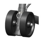
Adjust the height so that when the stand is locked in the lift position there is about 2 inches under the front tire. You want the <u>lowest height</u> that allows the wheel to clear the front fender when removed.
