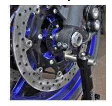
This stand is designed to lift from under the fork using the holes at the bottom of your fork tubes.
