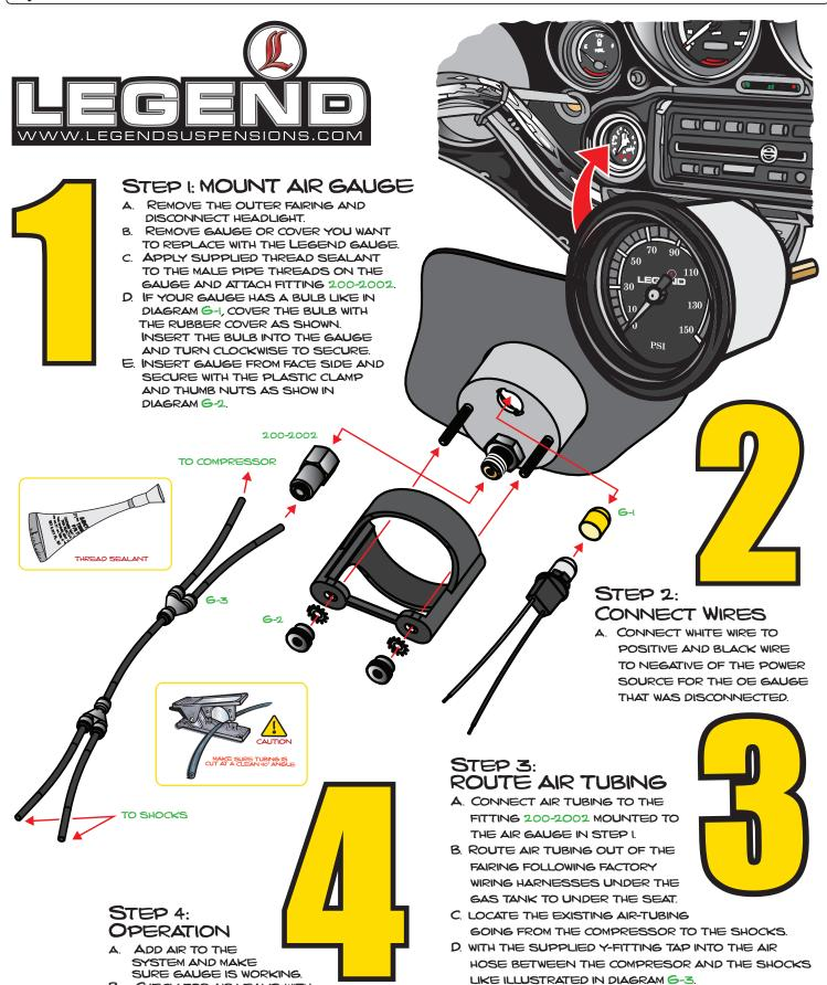
CHECK FOR AIR LEAKS WITH SOAPY WATER AROUND FITTINGS. RE-INSTALL SEAT AND OUTER FAIRING.
