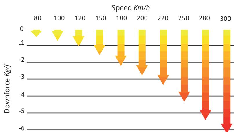
The Downforce that the spoilers generates raises potentially as the speed increases, at 300 km/h we get 6,3 Kg/f.
