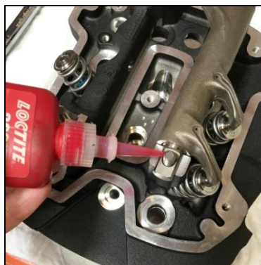
Loctite fine threads
