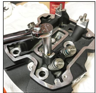
Torque stud to 4-5 Ft. Lbs
