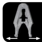
NOTE: The factory clips must be removed carefully! Using your thumbnails or a flat edge under each side, gently pry the 2 ends apart (as per the image) and pull up to release each clip from the stock grill. If you put a flat edge under one end only, the clip cannot release and you have a very good chance of breaking the clip.
