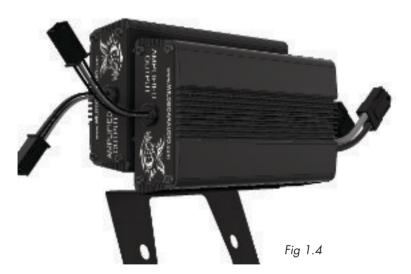
Step #10: Attach the amp's brown wire to the negative (-) battery terminal and the amp's red wire to the positive (+) battery terminal. The factory battery wires are also re-installed at this point. When attaching the power and ground wires, it is always a good practice to do the negative first. When the positive connector touches the battery, some sparking is normal. This is a function of the capacitors in the amplifiers charging up.
