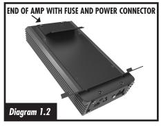
Step #2: Locate the main power harness that came with your amplifier and plug it into the amp.
