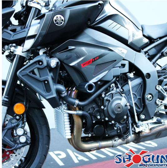
2. Remove right side bolt. Mount right side puck with (99-HB-SH12125080) Socket Cap 12 X 1.25 X 80 Main Engine Stud and torque down to the recommended OEM torque specifications.
