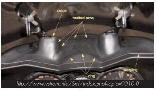
Photo above: Suzuki V-Strom upper dash cowl, a Parabolic Reflection created and made multiple ring burns, warping, and melted arc clusters. Owner was using a clear aftermarket screen with aftermarket brackets.
