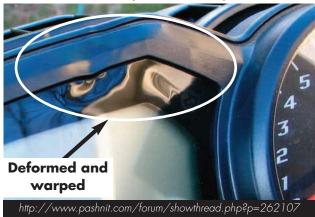
Photo above: Yamaha FZ1 instrument cluster deformed and warped. Owner was using a factory accessory touring windscreen.
