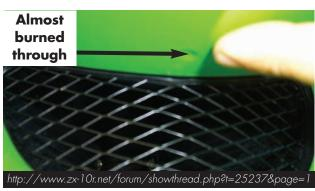
Photo above: Kawasaki ZX10R behind the instrument cluster, a Parabolic Reflection created and made a dimple in the fairing. Owner was using a clear aftermarket windscreen.
