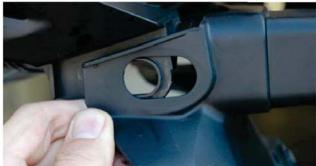
Install the Graves Fender Eliminator Kit onto the stock turn signal mounts.
