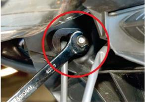
Remove the turn signal, metal insert and rubber insert. Repeat on opposite side.
