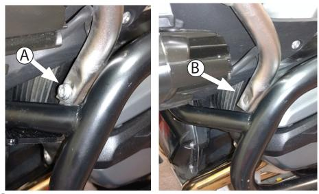
(A) Use T40 tool to remove the upper connector screw.(B) Remove the internal connector.
