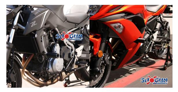
2. Remove Right side engine stud and mount Right side frame slider using 99-HB-SH10150180 Socket Cap 10 X 1.25 X 180 Main Engine Stud and 99-HN-LN10150 Lock Nut 10 X 1.5. Torque down to OEM torque specs.
