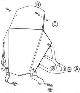
Install four (4) rubber grommets into headlight guard.(A) Use care to not rip the rubber. **!TIP** a dab of water will help them slide into place. Install rubber strip on rear of top edge.(B) Peel protective cover from polycarbonate lens. Install lens as shown with (6) supplied screws, washers, and nuts.(C) Install each screw loose first, then tighten down evenly.
