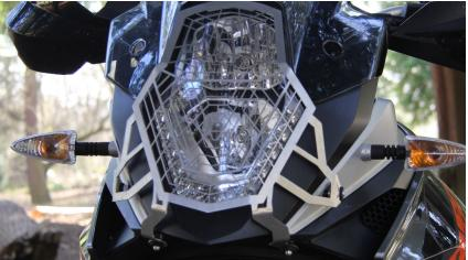
Install headlight guard. !TIP A dab of water on each ball stud will help it fit in place easier with less wear on the rubber grommets.
