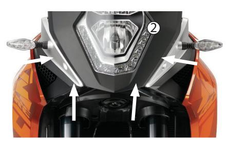
Use T30 Torx and remove four screws shown. One each just in front of turn signal, and two more under front lower edge of headlight guard (these are at a slight angle).
