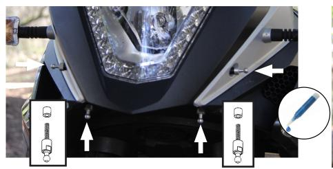
Apply a small drop of loctite to the threads of each ball stud. Thread in each upper ball stud on side panels near turn signals. Place one 10mm spacer on remaining ball studs and thread in to holes under front fairing as shown. Tighten to 5Nm
