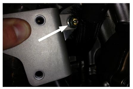
(8) Use 17mm socket and tighten the M10 screw to 49Nm. Bracket installation complete. Save the M8 x 25 socket cap screws for installing the crash bars.
