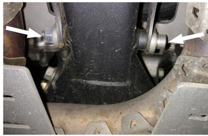
Screw the M8 x100 socket cap screw into the M8 lock nut and washer. Hold screw steady with 6mm allen tool, and use 13mm wrench
