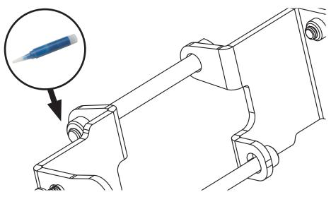
Place a drop of thread locker into the M10 captive nut on the Right bracket. Put the bracket in place and loosely screw in the M10 x 110 hex cap screw.
