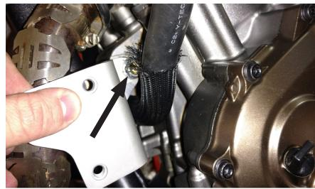
Insert the M10 x 110 hex cap screw with washer into the Left AltRider bracket. Place the bracket and screw in place and insert the screw through the Honda brackets and engine case, be sure the two OEM spacers are still in place.
