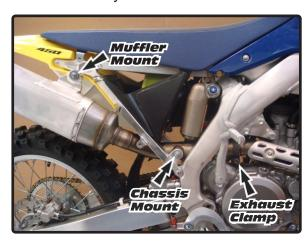
4. Remove the two header nuts and carefully remove the stock header. Inspect and replace exhaust port gasket if necessary.
