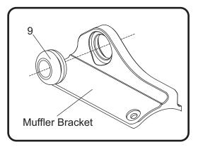
2. Install (No. 10) *ALS-010*, aluminum spacer into (No. 9) *Z1022*, rubber grommet as shown.
