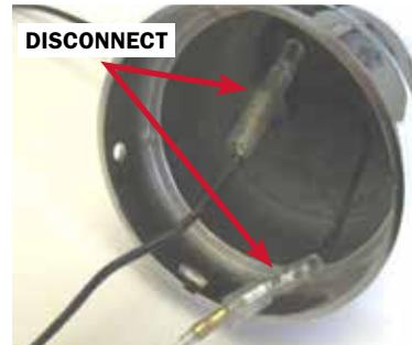
**STEP 4** Pull the glass housing out way from the light housing and disconnect the wires.
