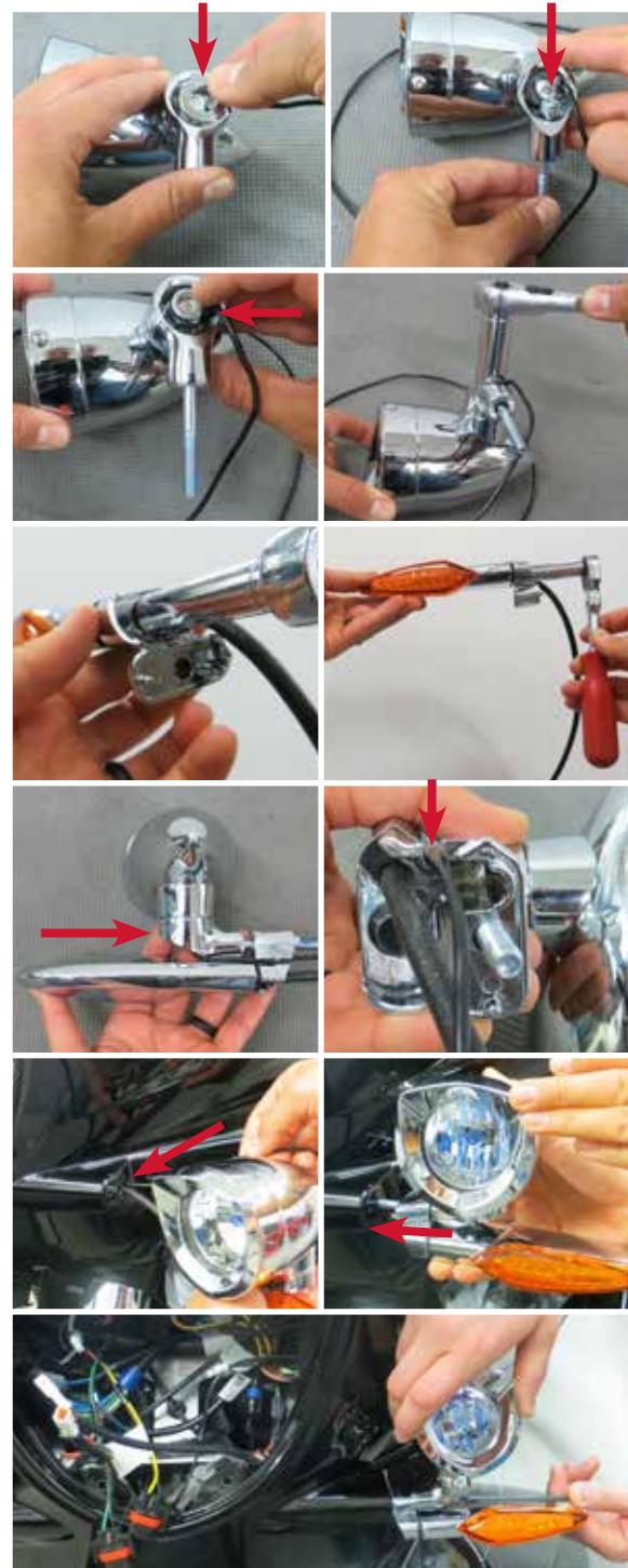
**STEP 19** Locate one 3/8-16 Locknut and attach it to the Driving Light Bolt. Align the mount as you would wanted it positioned on your motorcycle before fully tightening the Pivot Mount to the Driving Light.
