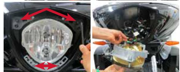
**STEP 5** Disconnect the Left Hand and Right Hand turn signal cables.
