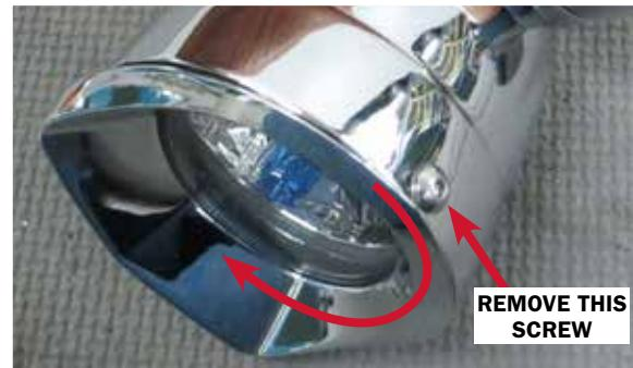
**STEP 2** Remove the light bezel by twisting the bezel counter clockwise and pulling the bezel outward.
