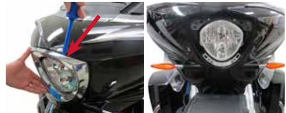
**STEP 4** Unscrew two top and bottom socket head cap screws from the headlight brackets.
