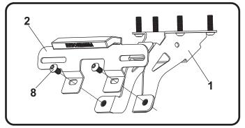
Install the stock plastic key hole cover onto (No. 1) 13100-FEBKT, fender eliminator bracket by inserting the key hole cover pins into holes A and B.
