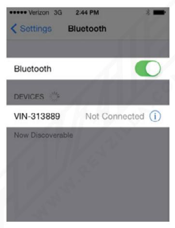
Ensure the Bluetooth toggle switch is in the "on" position. Then select the device label "VIN" ending with the last 6 digits of your motorcycle's VIN number. "Connected" will appear on the right side once the device has successfully paired with the Fuelpak FP3.
