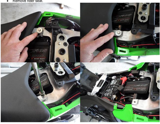
Remove rear side panels. There are several plastic fasteners, simply push in the center to release. Pull center back out and push back in to install.
