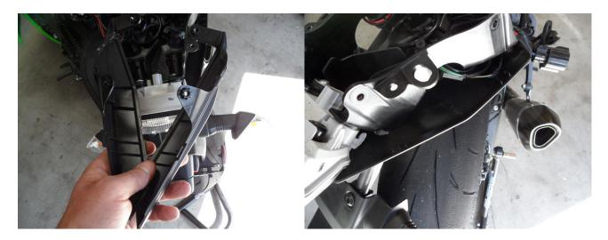
With the rear fender loosened and electronics unplugged gently pull the rear OEM fender out.
