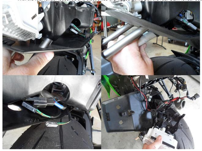
Install your Vortex Fender Eliminator Kit. NOTE: BUTTON HEADS MUST FACE UP WITH NO WASHERS!!! (Towards rider) There is not enough clearance between the storage compartment and under tail to use locknuts in this location. All washers go under locknuts. Make sure that the Vortex Fender Eliminator kit covers the two existing holes before tightening.
