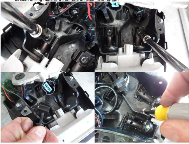
Remove smaller side panels attached to storage compartment. Note: There are nuts so you
