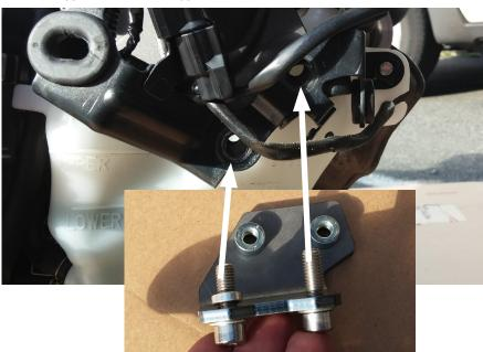
6 Install right front bracket as shown. Stack spacer in between AltRider bracket and Honda bracket. Attach with M8x 25 screws, torque to 19 Nm. Do not pinch wires.
