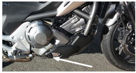
Remove plastic belly fairing(right and left side are connected). Use 5mm allen tool. Fairing has one screw on each side, and is also mounted via four rubber grommets. One grommet each side requires an outward pull on the fairing. Two forward grommets pull the fairing toward the front wheel.
