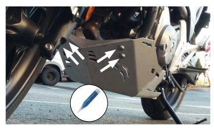
Attach four (4) front M8 flat head screws with finishing washers to front of skid plate. Screw most of the way snug. Use a drop of thread locker on each screw.
