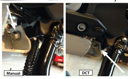
**Manual:** Use OEM Honda M8 x 18mm long bolt from step 2, plus the M8 flange nut. Attach the skid plate to the frame mount as shown, thread nut on then leave loose for now. 12mm and 13mm combination wrenches required.
