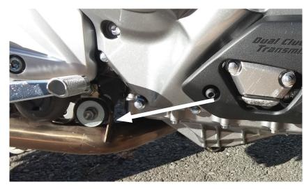
(5) Remove exhaust hanger bolt (under rear brake lever) as shown. Save for reinstall later.
