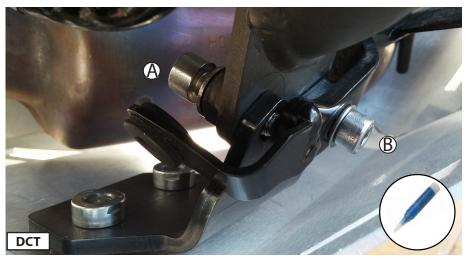
(8) **DCT:** Install left front bracket as shown. AltRider Bracket sits against frame, with DCT guard bar stacked on top. Apply loctite to these bolts. From backside, insert M8 x 20 bolt (A) and tighten to 10Nm. This acts as as support pin to the AltRider bracket. Use M8 x 25 bolt from outside (B), through both DCT bar and altrider bracket. Do not fully tighten this bolt yet.
