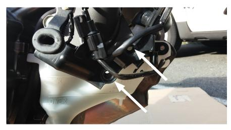
② Use 12mm wrench, remove two M8 bolts from from right side brackets on frame mount as shown. Leave brackets in place. Save the bolts for use later.
