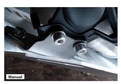
Manual Transmission: Install left front bracket as shown. Note orientation of bracket. Attach with M8 screws (one M8 x 25, one M8 x 20), tighten to 19 Nm.
