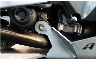
(12) Attach the left rear mount of the skid using the exhaust hanger bolt. (12mm socket). Leave loose for now.
