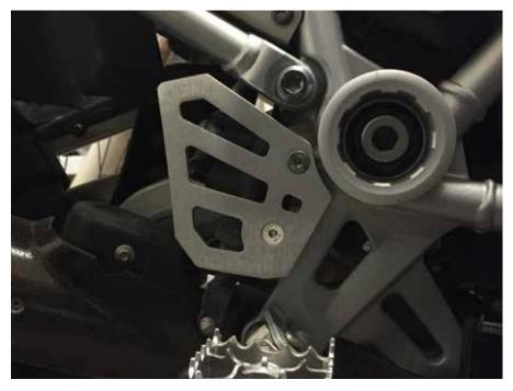
Apply two drops of thread-locker to the ends of the (2) M6 flat head fasteners provided. Install the new guard with the spacers positioned on the M6 flat heads, BEHIND the guard.
