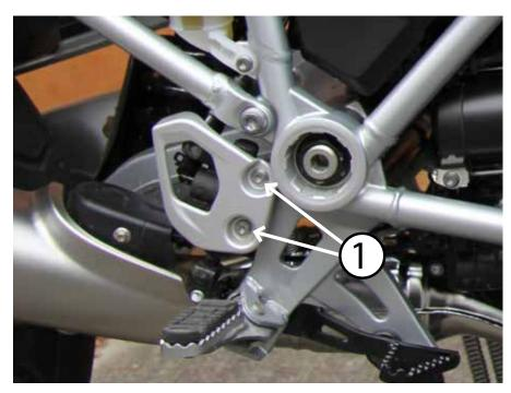
Remove the (2) T30 torx fasteners from the rear brake master cylinder assembly. Remove the OEM guard and the torx fasteners.
