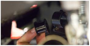
14. Before you run the bike, clean off all fingerprints and dirt, as any oily residue will etch the metal and become somewhat permanent when the system gets hot. Run the bike and enjoy. It is normal for some white smoke to appear the first time you start the bike. This is packing/manufacturing oil from inside the pipe burning off. Check for gaps or leaks. If you find a leak, a little high temperature silicon sealant should fix it. After 50 to 100 miles, recheck all fasteners for tightness.
