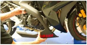
Remove OEM muffler assembly. Muffler mounting bolt will be re-used with TBR muffler.
