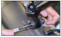
Remove header assembly including butterfly cables, loosen radiator bolts for better access.
