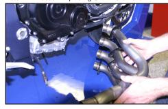
11. Attach muffler to TBR slip system using the supplied X-ring, 6x20mm socket head cap screws and lock washers that are provided, leave loose for now. Slide rubber lined muffler clamp and barrel clamp on and install to bike.
