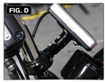
The Power Vision module may be mounted to the bike's handlebars using Techmount hardware.
