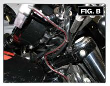
Route the Power Vision cable away from any moving or hot parts.
