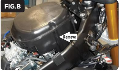
2 Remove the airbox (Fig. B).
