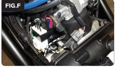
Plug the pair of the 3-pin connectors on the PCV wiring harness in-line of the bike's TPS and the stock wiring harness (Fig. F).
