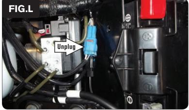
Locate and unplug the stock connector for the bike's Rear O2 Sensor (Fig. L).
