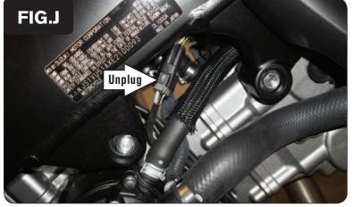
1 Locate and unplug the stock connector for the bike's Front O2 Sensor (Fig. J).
