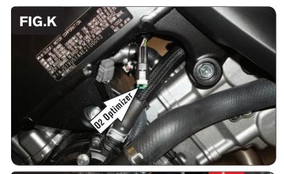
12 Plug one of the supplied O2 Optimizers into the bike's wiring harness in-place of the stock Front O2 Sensor (Fig. K).
