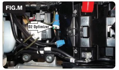
14 Plug the other supplied O2 Optimizer into the bike's wiring harness in-place of the stock Rear O2 Sensor (Fig. M).
