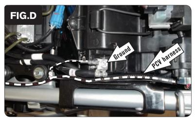
5 Secure the PCV ground wire with the small ring lug to the negative (-) terminal of the bike's battery (Fig. D).
