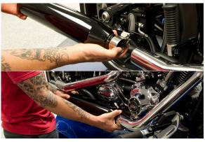
TBR mufflers are specific to front and rear cylinders and are marked accordingly.
