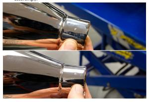
Remove OEM joint clamp and install onto TBR inlet. Install TBR slipon onto OEM head-pipe.
