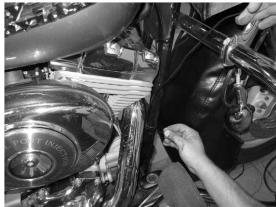
Tighten temp sensor with a 3/4" wrench
