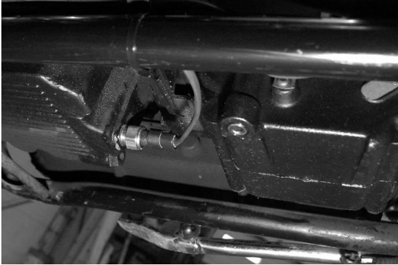
Installed oil temp sensor and harness plug
