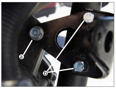
Pre-2008: Remove both (a) and (b) bolts. Remove bolt (a) using a 14mm socket and wrench, save this bolt. Remove bolts (b) using a 13mm socket and 12mm wrench. 2008-Newer: leave oem brackets in place unless you have puchased the KL08-1/2-1200 kit with upgrade brackets.
