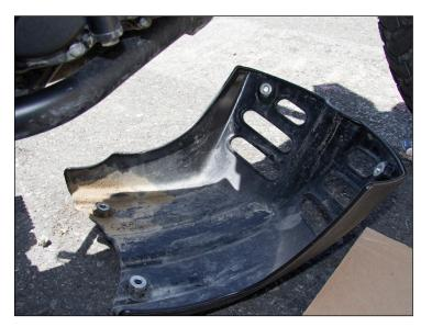
Remove OEM skid plate by removing the (4) 6mm bolts with an 8mm socket. Set these screws aside however you will not need them any longer.
