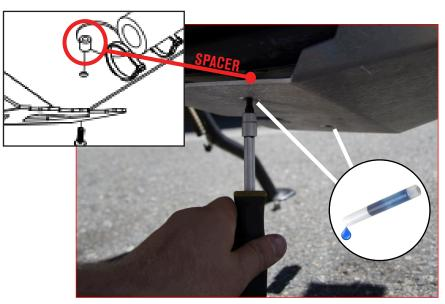
On the bottom of the skid plate start the (2) M6 x 22 flat head screws. Add the (2) 13mm aluminum spacers and a drop of thread locker to each screw before inserting it into the threaded bosses on frame rail. Now you can tighten all (4) M6 flat head screws.
