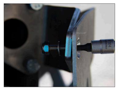
Hold skid plate up to front brackets and start the (2) M6 x 16 flat head screws in the front of the skid plate. Add washers and nylock nuts. Do not tighten all the way.
