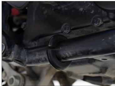
All years: add (4) of the rubber split-ring grommets to each side of the frame rails directly under the engine and wrap (1) zip-tie around each grommet with the zip-tie laying inside the slot of the grommet. You can use oil as lube to help set zip-ties into grommets. There should be a total of (8) grommets installed on the bike.
