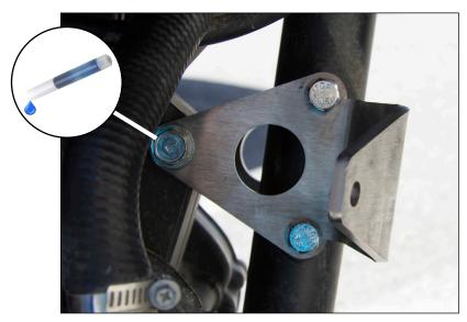
Pre-2008 and upgrade: Install stainless steel brackets used the OEM M10 engine bolt and nut, and (2) AltRider supplied M8 x 85mm hex head bolts, washers, and nylock nuts. Completely tighten all three of these bolts.
