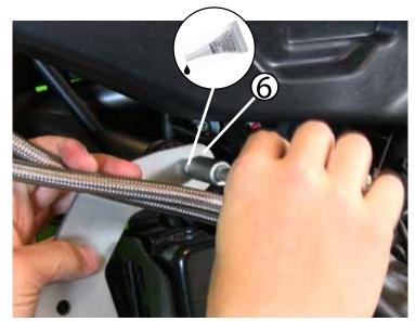
Using a 10mm socket and driver, remove the left side radiator mount bolt. Now put the crash bar bracket in place as shown and use (2) M6 x25 fasteners to mount the bracket. Do this on both sides and leave it just loose enough to move the bracket.
