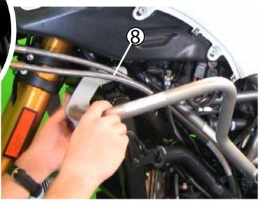
Rotate the bar up as shown. Once the bar lines up with the mount bracket, tighten the radiator mount bolts to the OEM torque spec.
