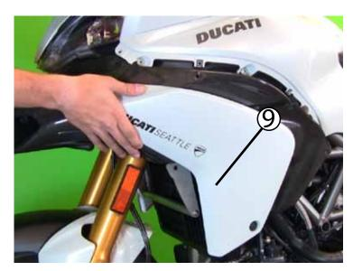
As when removing the plastics, be very careful when putting them on to not force the fit. Don't forget to re-seat the post in the grommet at the oil cooler, and don't forget to plug in the air temp sensor!
