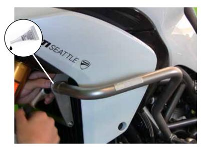
Using a 15mm socket, tighten the hex cap fasteners into the crash bars on both sides. turning the front wheel can give you better access for this step. **Don't forget thread locker!**
