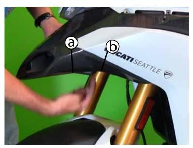
Before removing the fairing/beak, you need to: (a) release the nose from a grommet just in front of the oil cooler, and (b) unplug the air temp sensor on the riders right side of the nose, follow the intake until you see the sensor plugged in.
