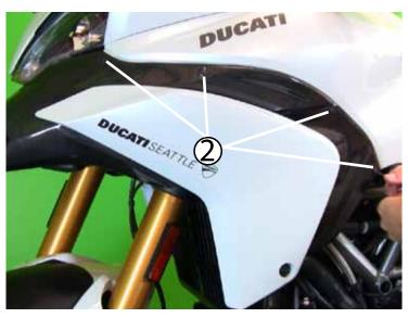
Using a 3mm allen tool, remove the (4) fasteners holding the fairing and beak in place. Keep your hardware in bags or trays to keep it organized. Do this on both sides.
