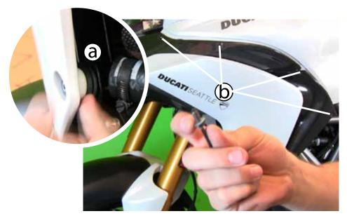
(a) Push rubber grommit back into its radiator bracket on both sides. Some spray lubricant can help here. (b) Using a 3mm allen tool, insert all the fairing fasteners. Don't forget your nylon washers if you have the S model w/carbon fiber.
