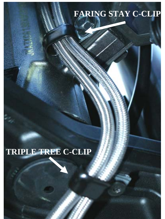
B. C-clip at Faring Stay and C-clip at Lower Triple Tree
