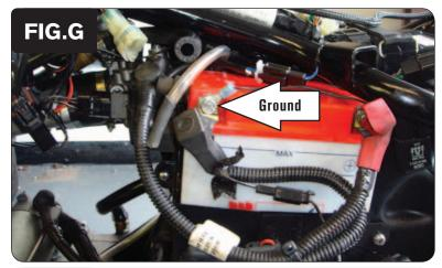
Secure the ground wire of the PCV wiring harness with the 6mm ring terminal to the negative terminal of the bike's battery (Fig. G).
