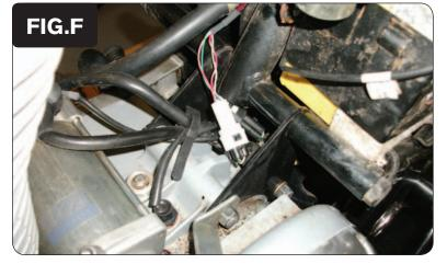
Plug the pair of PCV wiring harness leads with BROWN colored wires in-line of the stock Crank Position Sensor connectors (Fig. F).
