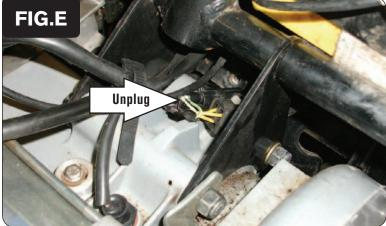
11 Locate and unplug the bike's Crank Position Sensor connector (Fig. E).
