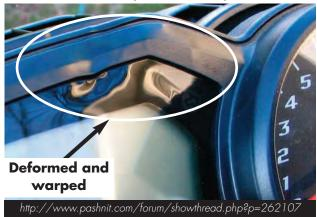
Photo above: Yamaha FZ1 instrument cluster deformed and warped Owner was using a Yamaha accessory touring windscreen.
