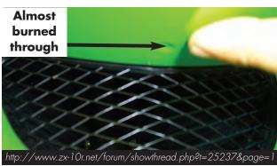
Photo above: Kawasaki ZX10R behind the instrument cluster, a Parabolic Reflection created and made a dimple in the fairing. Owner was using a clear Puig windscreen.
