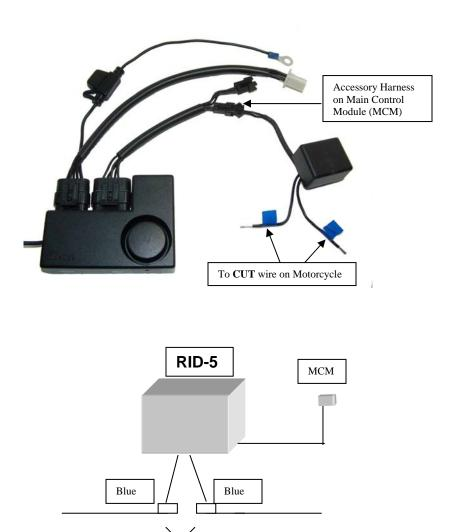
**Note:** The RID-5 will also add an Ignition disabling feature, and will prevent unauthorized starting of the engine automatically when the system is armed.
