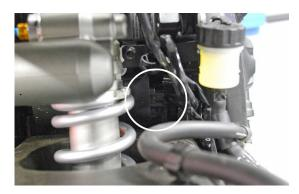
2. Unplug the servo connector. Remove the EXUP servo from the motorcycle.
