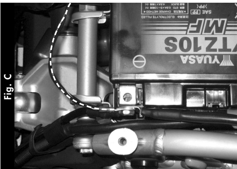
4. Connect the ground wire from the PCIII to the negative side of the battery (Fig. C).
