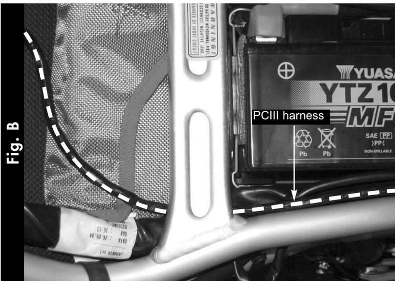
3. Route the Power Commander harness underneath the right side of the frame rail towards the front of the bike (Fig. B).
