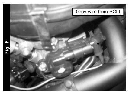
Unplug the connector from right outside injector (Cyl 4). Plug the PC connector with the BLUE wire inline with the bike's harness connector and the injector. Continue for Cylinder 3 with the PC connectors with the GREEN wire, for cylinder 2 with YELLOW, and cylinder 1 with the ORANGE wire.
