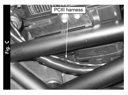
Continue routing the PC harness along the inside of the Bike's main harness, underneath the fuse box and toward the throttle bodies.
