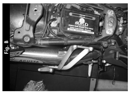
Route the Power Commander harness along the right inside of the subframe towards the front of the bike. Attach the ground wire from the Power Commander to the negative side from the bike's battery.
