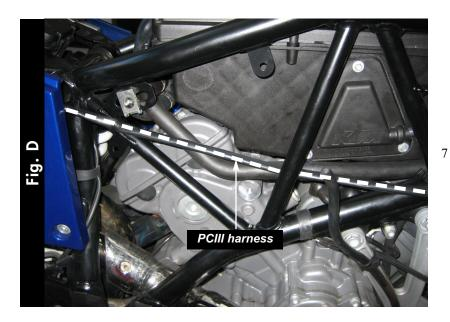
Route the PCIII harness inside the right hand side frame tubes (Fig. D)
