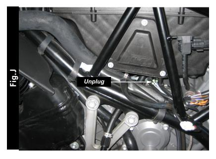
Locate the connector for the rear cylinder O2 sensor. This connection is located on the left hand side of the air box (Fig. J).
