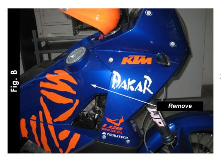
Remove the right and left hand side panels and fuel tanks (Fig. B).
