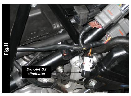
Plug the Dynojet 02 eliminator into the stock wiring harness (Fig. H).
