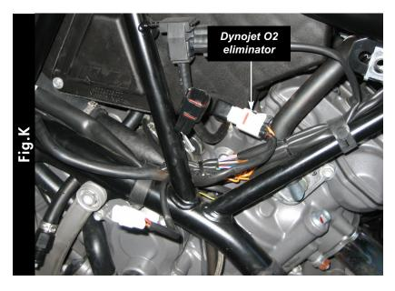
17 Plug the Dynojet 02 eliminator into the stock wiring harness (Fig. K).
