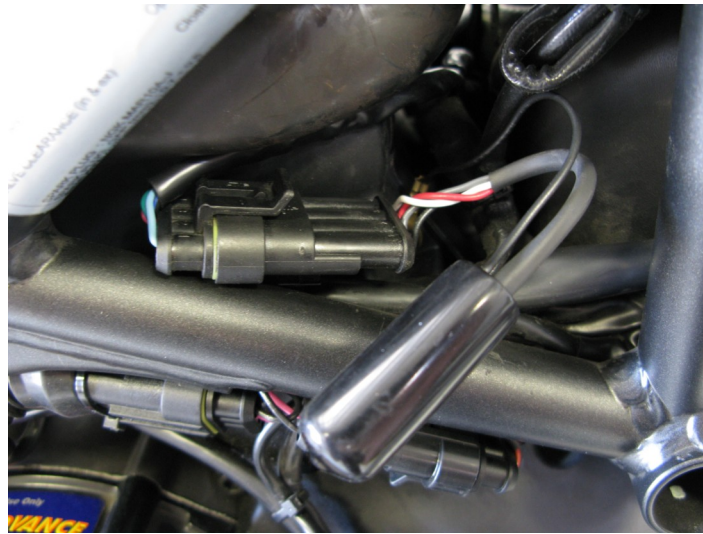
Bazzaz O2 eliminator installed
