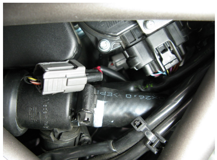
Bazzaz harness installed in-line
