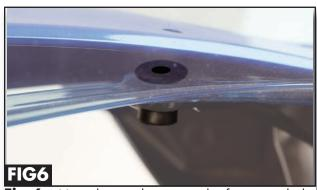
**Fig 6.** Mate the windscreen to the fairing with the flange of the well nut facing under the fairing. Make sure that the well nut fits back into any brackets it did during your removal in step 3.
