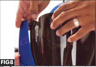
Fig 8. Holding the windscreen in place with one hand, begin threading the new bolts through the fairing holes into the well nuts. Start this at the bottom and work upwards in pairs side to side.
