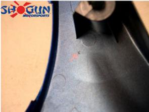
9. Using a small drill  $\frac{1}{4}$  inch or so drill a pilot hole in the body from the inside out. Remount bodywork and double check the hole location with the spot tool still inserted (arrow in picture below is pointing to spot tool). With pilot hole cut and on center, remove body and disassemble panel to prep for cutting.
