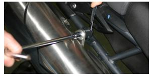
Loosen pipe joint clamp.
