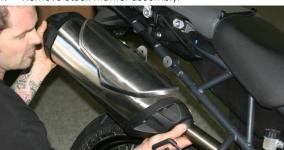
Attach TBR slip tube to TBR muffler using the 2 piece X-Ring and 6x14mm socket head cap screws with lock washer that are provided. Leave loose enough to make some adjustments on the motorcycle.
