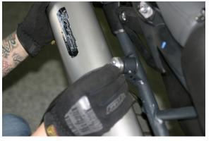
Install rubber lined muffler support strap and attach using OEM hardware.
