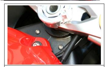
This photo shows the bike with the stabilizer kit removed and the holes plugged with stainless bolts. Black bolts would blend with the frame and not show.
