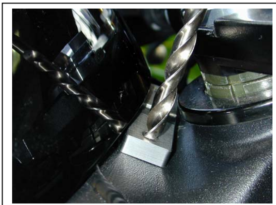
Some models allow drilling without removing the triple clamp. Keep the drill perpendicular to the frame being careful to drill a clean, straight, hole.
