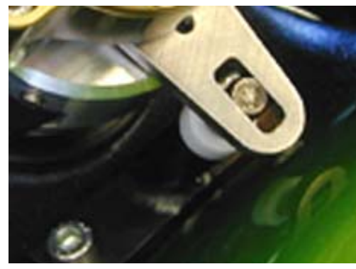
Tower pin location / not binding in slot
