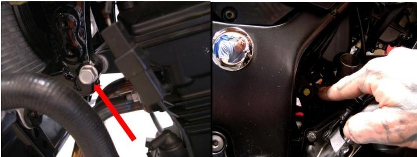
5. Make sure the vehicle is in a fixed secure position. With a standard floor jack **support** the engine enough to remove engine studs. To help prevent scratching of any kind or damage to the bike when lifting we use a small piece of soft wood or a plastic puck on the jack pad. With jack secure and in place remove each front and rear stock engine studs.
