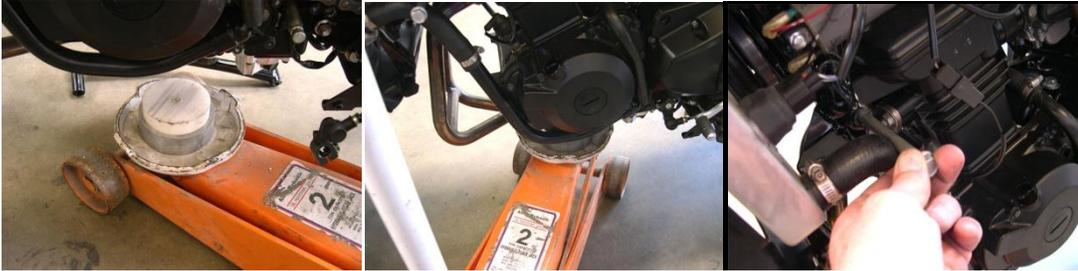
6. Loosely mount the left side rail passing the (99-HR-TH3/8-16 x6 11/16-R) 9/16 X 160 welded threaded rod in the rear through the Shogun rail towards the right side of the bike. Use the (99-HR-TH3/8-16x9 15/16-F) 9/16 X 245 welded threaded rod in the front. Pass it through the Shogun rail towards the right side of the bike. When installing the front rod lightly press down on the radiator hose so the bolt can pass.
