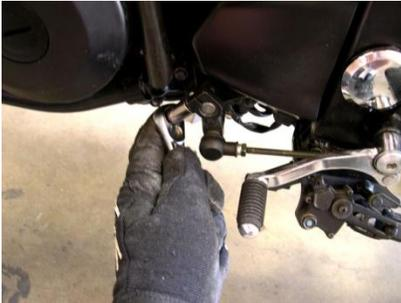
12. Mount left and right side sliders using 99-HB-SH10125080 Socket Cap 10 X 1.25 X 80 (Holds puck to offset) 99-HW-M10WASH Washer M10 Zinc Plated 99-LN-LN10125 (one washer goes under the head of the bolt, one goes under the Hex Lock Nut) Hex Lock Nut 10 X 1.25 (Left side slider longer than right) Torque down to 40 ft lbs.
