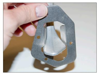
Slide the top plate over the foot of the side stand as shown. At this angle, it will easily clear the 'heel' of the foot.
