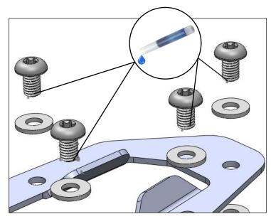
Apply one drop of Loctite to the last couple threads on all of the fasteners, then assemble the large sidestand foot on to your sidestand. Be sure to place (1) washers between top and bottom plate. (reference the exploded view on pg1)
